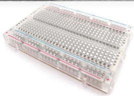
Breadboard: Wires plug into its sockets.
