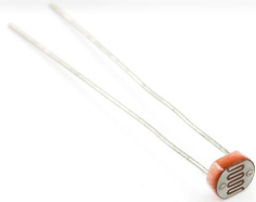
Photocell: Changes resistance with light.
